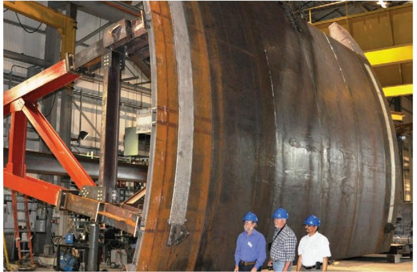
Gates were fully assembled in the shop and components match marked to facilitate field assembly and installation.
