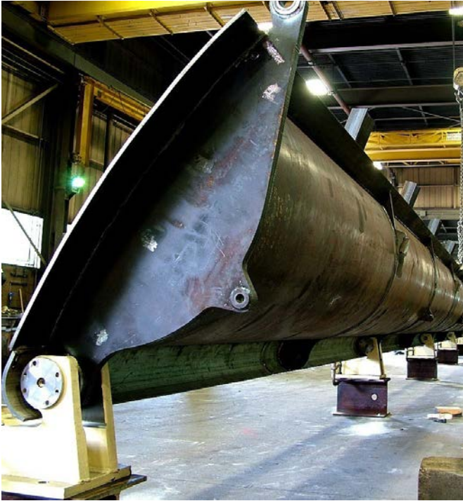
Lake White State Park Dam, Ohio – Pelican® Crest Gate (68' x 4')
