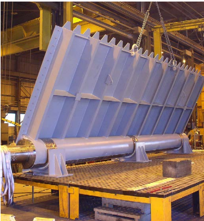
Jacob Fork Pump Station, North Carolina – Bascule® Crest Gate (25' x 10')
