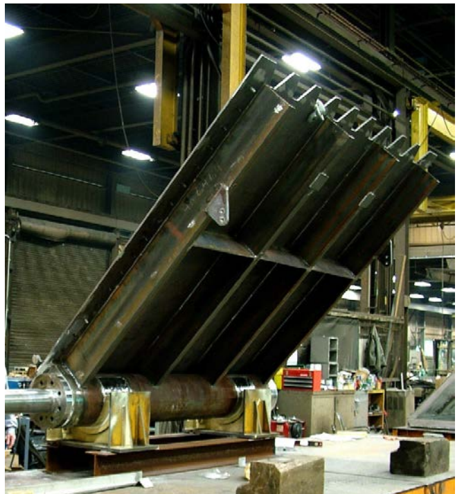
Olin Corporation McIntosh Plant Site, Alabama – Bascule® Crest Gate (10' x 8')
