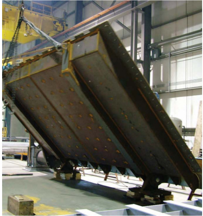
East Fork Shoals Creek, Illinois – Bascule® Crest Gate (25' x 11' 8")
